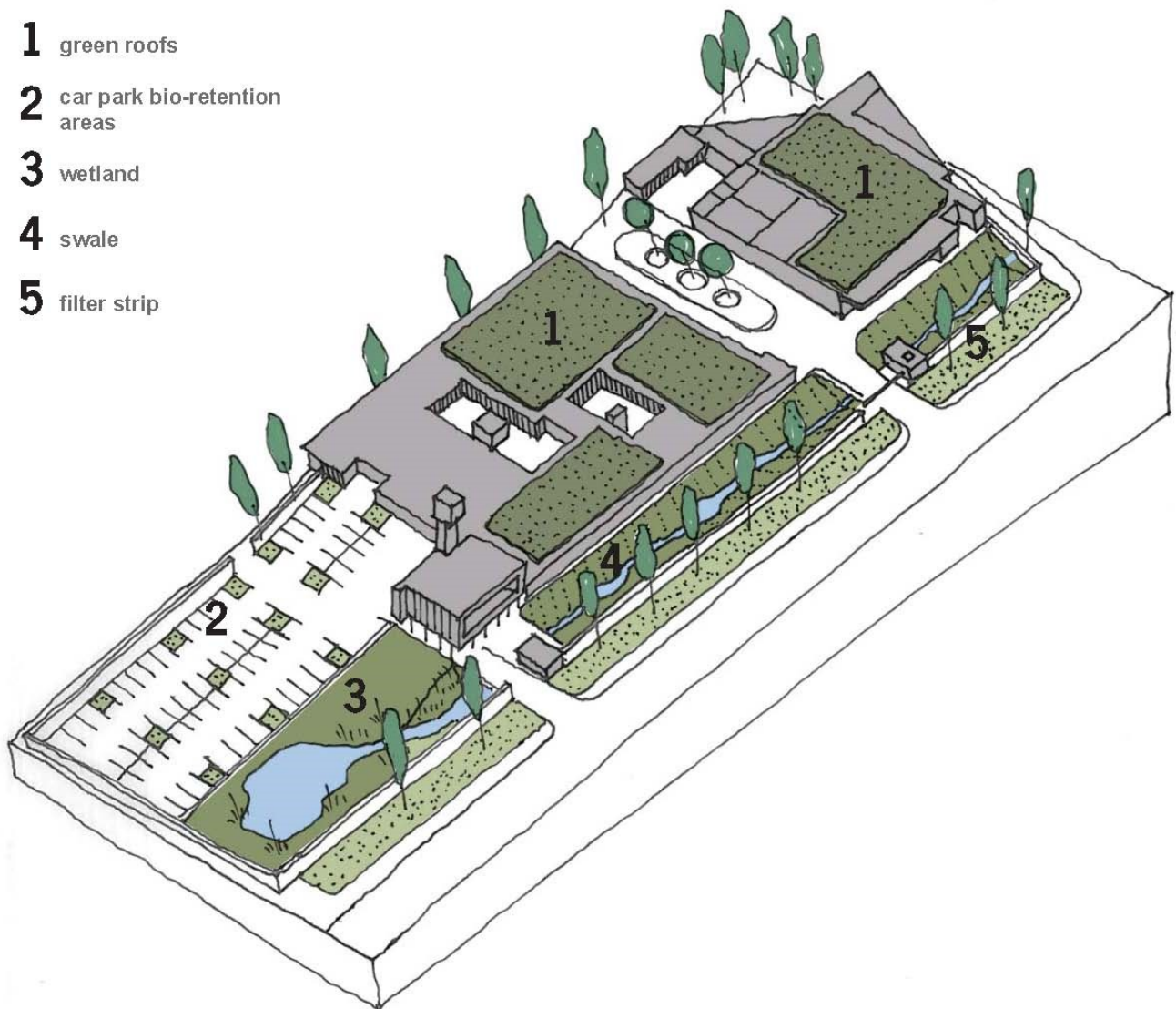
Figure 6.18 : Incorporating SuDS on industrial sites
