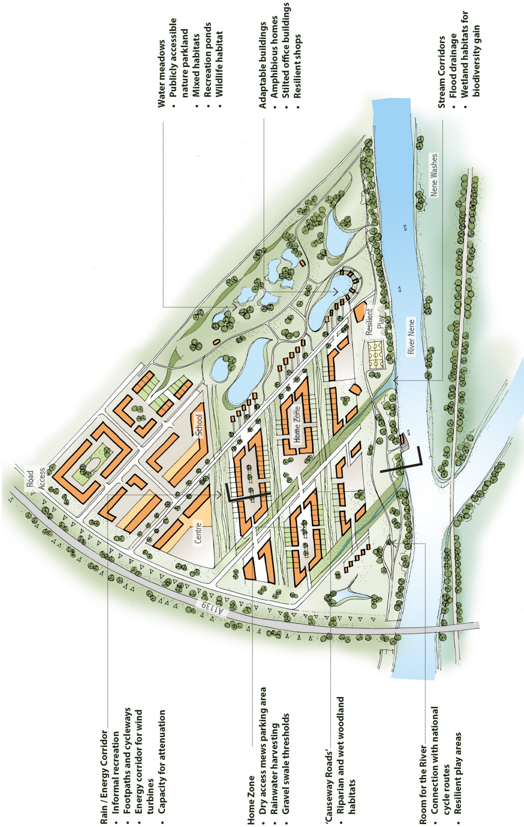
Figure 5.2 : Middle river catchment development ©BACA Architects
